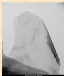
TEM images of the sample after 1 min (left) and 120 min (right) of CCVD reaction time. \text{CH}_4:\text{H}_2 = 2:1 , Temp.: 950 °C
